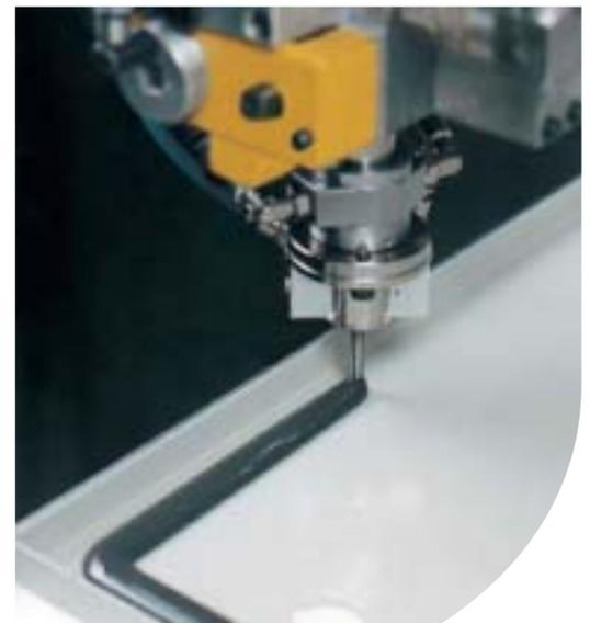
production scraps, the foaming phase must be robotically (not manually) assisted.
