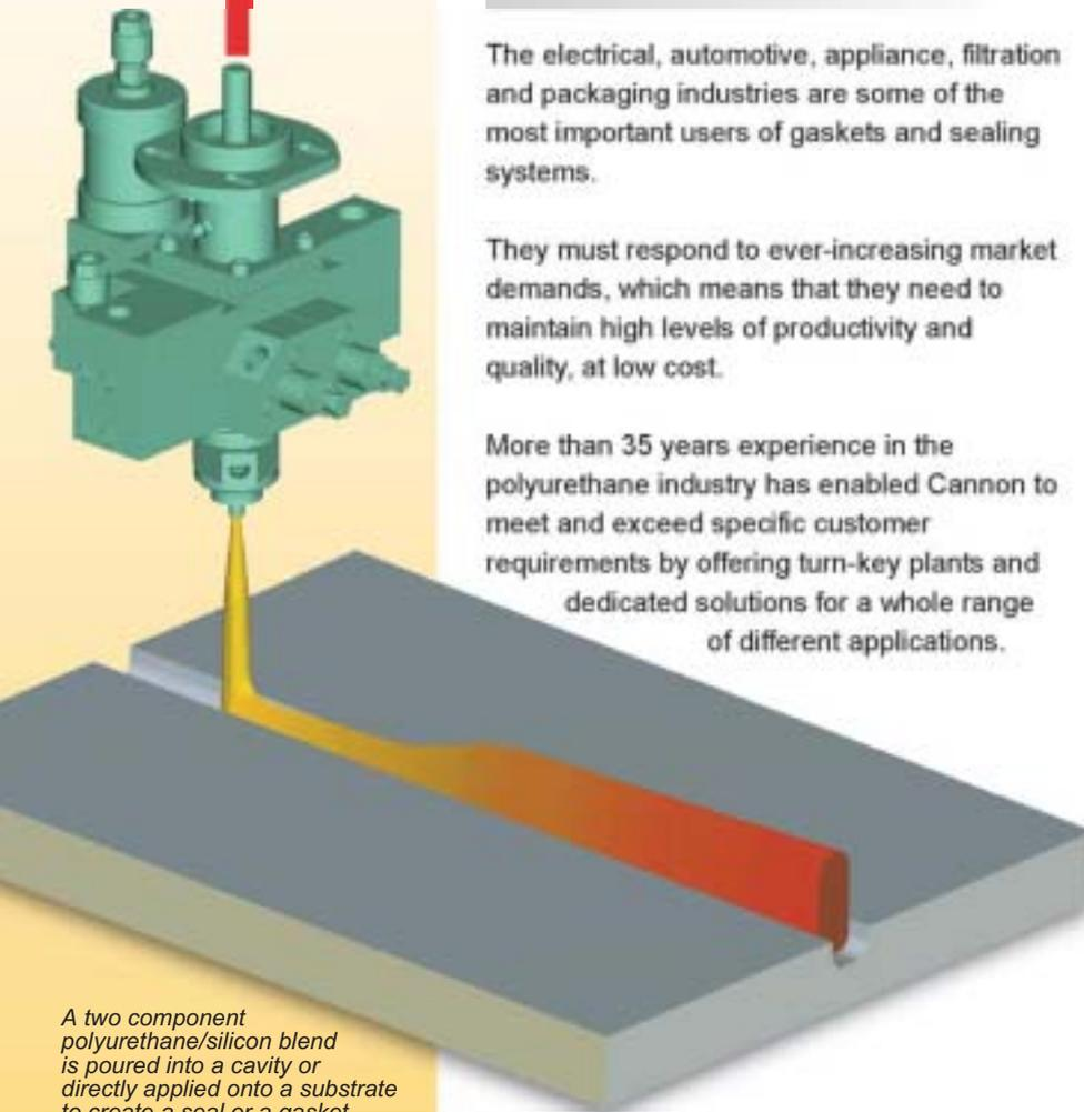
*A two component polyurethane/silicon blend is poured into a cavity or directly applied onto a substrate to create a seal or a gasket.*
