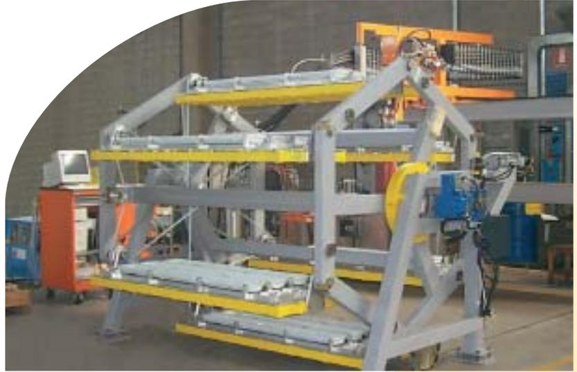
*Six positions drum for lamp handling.*
