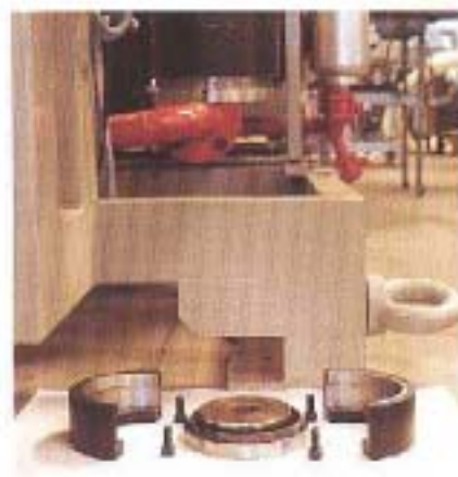
Fig. 7 - Cylinder in maintenance position for seals replacement.
