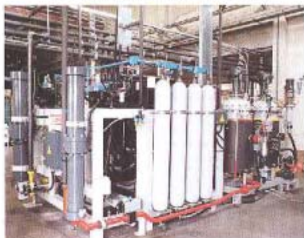
Fig. 13 - "HE-System 700 Booster 25/13" accumulator machine for output rate up to 700 kg/min.
