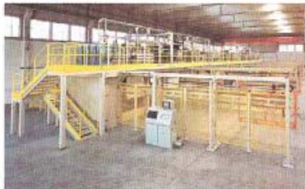
Fig. 12 - Multi-heads plant for glass encapsulation.
