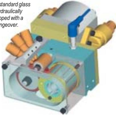
At the same time in a typical foaming cycle, the solid component is metered and fed by the upper section of the head through a specially designed chopper hydraulically controlled and assisted by pressurised air. The process is completely automated and each single step is monitored by a sophisticated control system to ensure constant process repeatability and component ratios.
