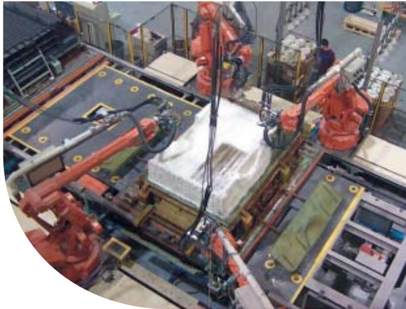
Sophisticated InterWet multihead system for the production of glass fibres PU reinforced automotive exterior body parts.
