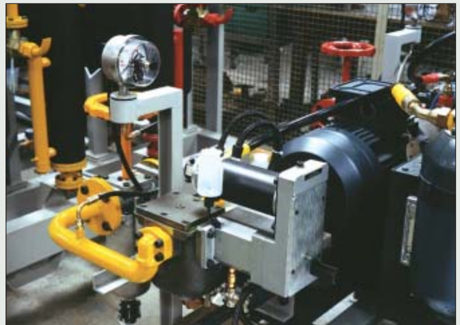
High pressure pump with closed-loop control.
