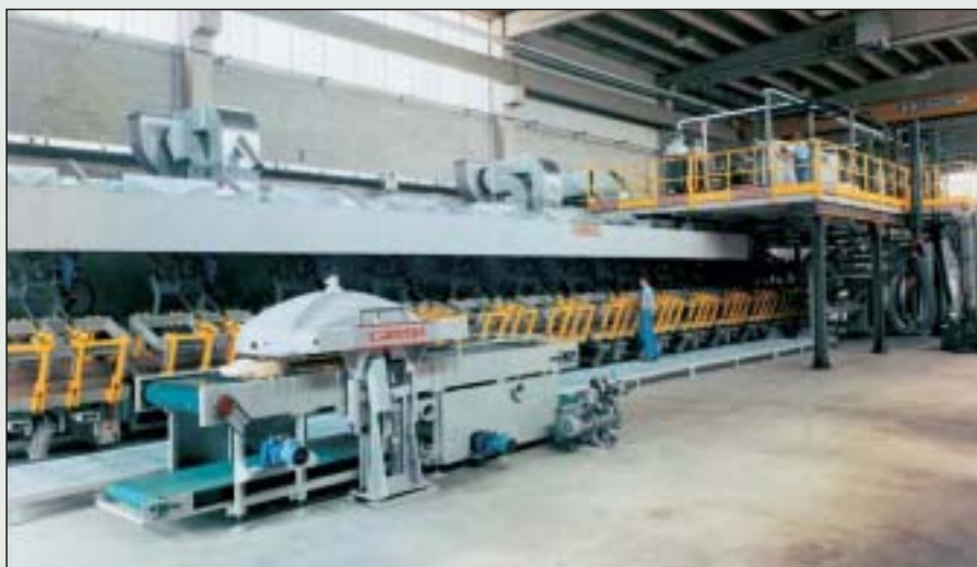
Turning tables for automotive seating production.
