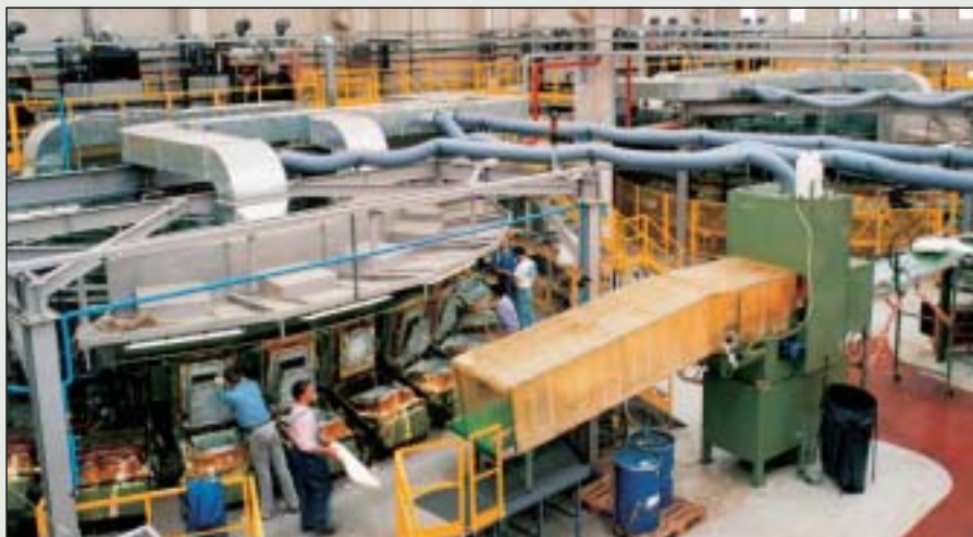
Turning tables for automotive seating production.
